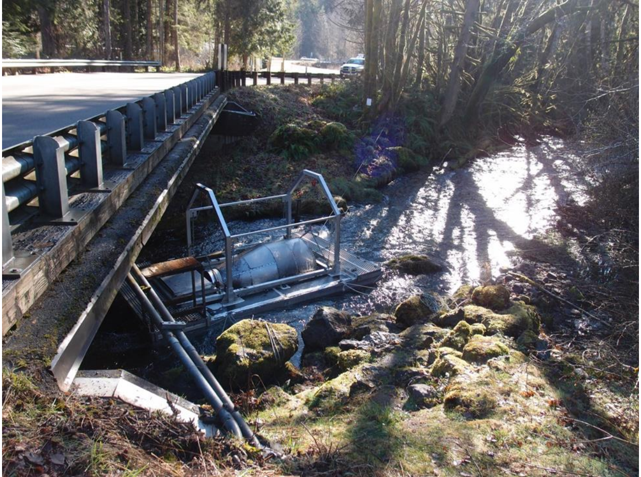
Figure 5. Indian Creek 4' screw trap fishing spring 2014.
